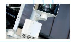
LOC.id-capable construction site systems (beacons) acoustically indicate the way through the construction site bypass by emitting two temporally staggered acoustic signals of different timing at the entrance of the bypass, which are clearly different from usual ambient sounds.
